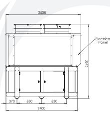
Note: 8G R32 Series heat pumps and chillers are not suitable for indoor/plant room installations without air quality monitoring and ventilation due to mild flammability.
